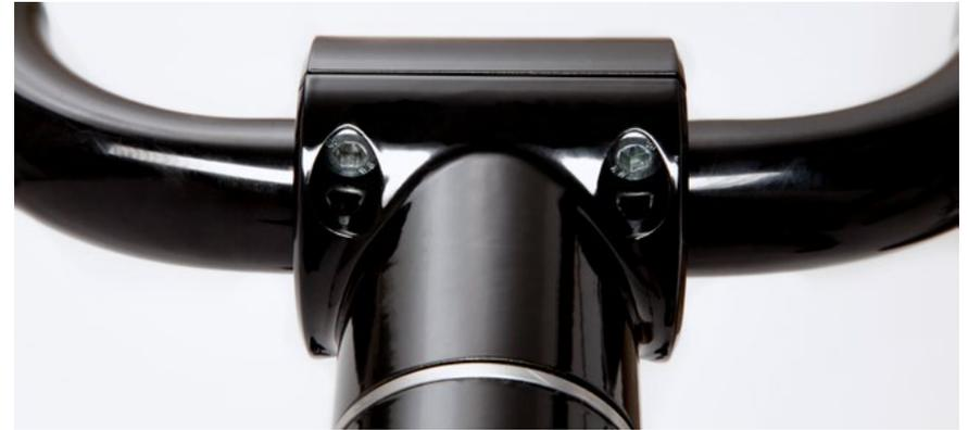
2. After adjusting the handlebars, carefully tighten the four screws again. To achieve the required clamp tension between the handlebars and the handlebar clamp, the screws must be tightened to a torque of 15 Nm.
