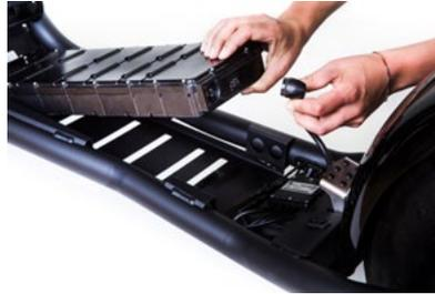
You can now charge the battery in an ordinary household plug socket (220/230 V) using the charger supplied with the SCROOSER.
